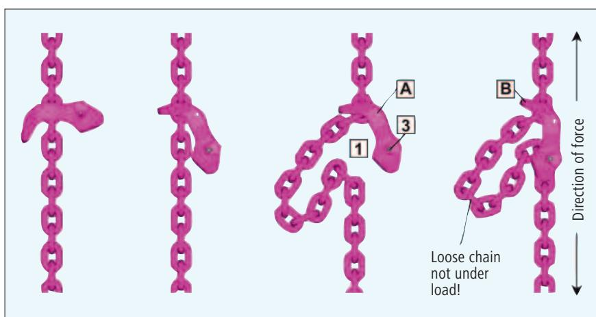
1. Attach loose chain strand through cross of IMVK and secure by hammering the sleeve pin **A** in.
