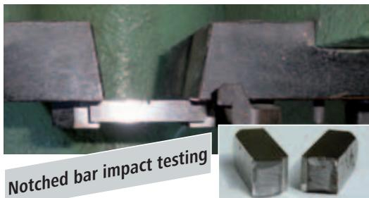
With an impact test, it can be shown if the chain has enough toughness when it is exposed to severe conditions.
