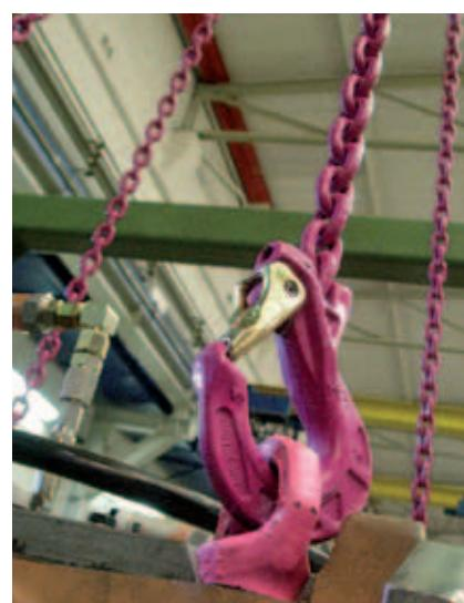
Consisting of a forged safety latch, triple-coiled corrosion resistant double-leg spring and a retaining pin.
