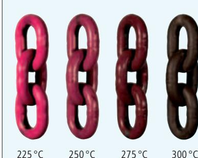
The special ICE-Pink-Powder Coating shows the effects of temperature in which the chain can be safely used. It is prohibited to use the ICE-Pink chain in temperatures of more than 300 °C. This is clearly displayed by ICE-Pink colour turning brown-black.
