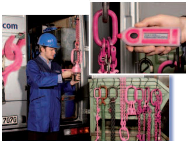
Regular inspections of lifting applications are an essential requirement to ensure the highest standard of safety is met. Dated methods of inspections involve copious amounts of paper work and time consuming manual processes.
